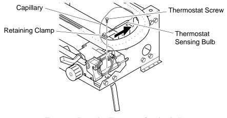
Figure 28 - Removing Thermostat Sensing Bulb
